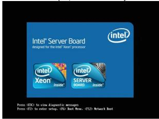
1) Press "F2" to enter BIOS on boot and press " $\rightarrow$ " to switch to "Advanced".
