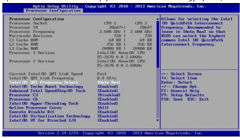
4) Press "Enter", and then " $\downarrow$ " to modify the option of "Enabled", and apply.
