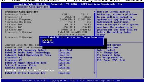
5) Press"  $\downarrow$ " to the "Intel(R) VT for Directed I/O" option, and modify the option to be be "Enabled".
