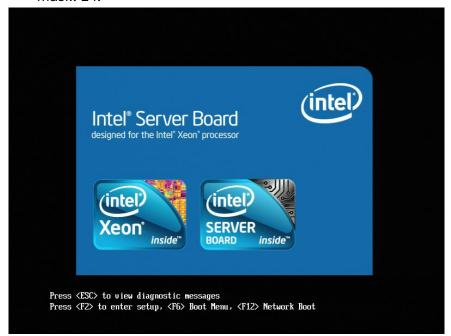
1) Press "F6" to enter the boot menu. After entering Boot Menu, press " $\uparrow$ " and " $\downarrow$ " to select the start device, and then press "Enter" to confirm.
